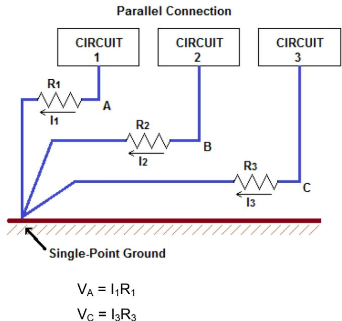
What NITEK can provide is a means of re-directing the coupled energy from the lightning away from the IP devices, both outside and inside. Initially, we'll look at the equipment mounted in the elements, where it's most likely to encounter dangerous voltages/currents. The image on the right depicts the basic surge protector provided by NITEK combines the functionality of a single-point ground with surge protection devices, which conduct only when a surge is present on the lines.
