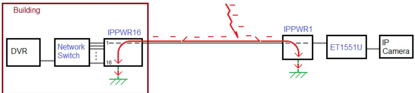
As the lightning strikes the ground, a surge is built-up in the cabling and travels towards both the camera and the building. During normal operation, the surge protection allows the Data/PoE+ (58Vp-p) to pass through with-out affecting the data or power. But during a surge, a path to earth ground is created allowing the surge to be directed away from the other devices.
