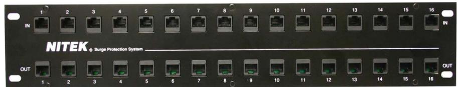
IPPWR16 is rack mounted in a standard 16 inch rack (2RU height). The IPPWR16 allows a surge to be routed to ground, by the use of a heavy duty single-point connection, and clamps the protected equipment video inputs to a minimum voltage.
