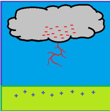
In the event of negative cloud to ground lightning, the ground is positive with respect to the charge built-up in the cloud. The initial strike (always taking the path of least resistance) creates a path using stepped leaders from the cloud to the ground (see figure on the left). As the cloud leaders approach the ground, ground leaders reach up seeking a path to complete the circuit (figure on the right).
