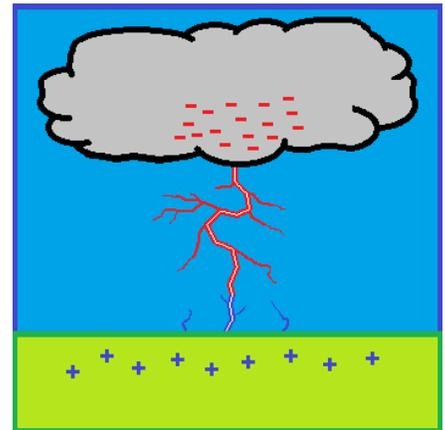
Once the circuit is closed, the full current (somewhere between 20,000 to 100,000 Amps) of the up-ward return strike flows, with a time duration between 20 and 90 micro seconds. Most of the energy of the strike is used in the creation of the pathway (between the cloud and the ground), heat energy and light. In the photo to the right, near the bottom, the ground leaders are visible, as-well-as the return strike.
