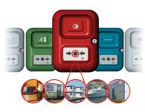
Once activated the Alert Point will emit a 102 dB(A) alarm, an activation flag drops into view and the built-in LED facility flashes red. Any external connected devices will be activated. The Alert Point can be easily reset with a special key, ensuring that the unit is quickly operational again. An override facility can silence the alarm until the Alert Point can be reset.
