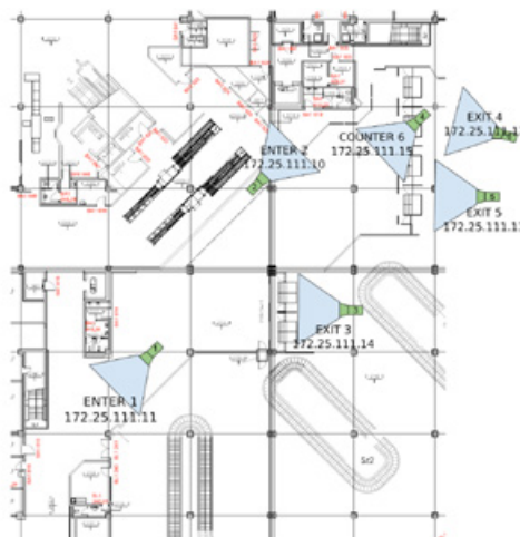
Face recognition camera setup at Budapest Airport to measure waiting times
