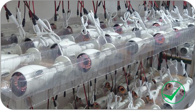
12-hours aging test after QC, ensure high quality & Long-life products
