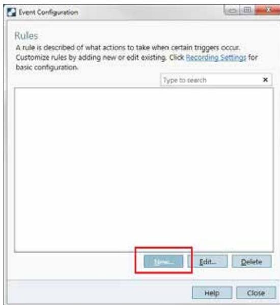
7. There are 4 main steps to create an event rule within ACS. These include the trigger for the event (Input), the resulting actions required (Output), the schedule for the event, (when is it active) and finally the naming details of the event for reference. Click 'Add' to create the first input trigger.
