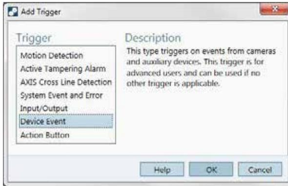
9. The device trigger will always be the View Area 0 camera and not any of the user created View Areas (i.e. 1 and above). This is because the ACAP is linked to the main View Area 0 within ACS. If any of the user View Areas are selected here then an error will occur. The selection of which virtual cameras to display is done in the next section.
