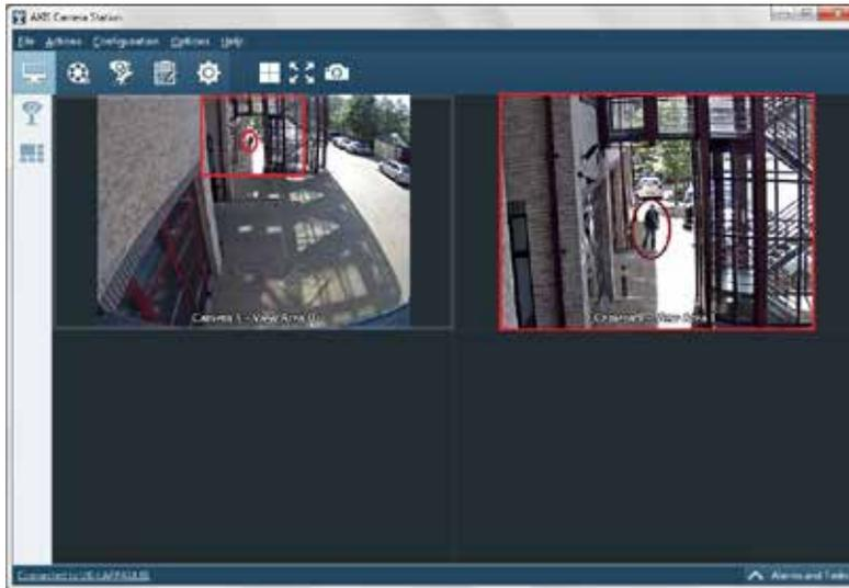
The image on the right is simply a virtual camera created by cropping the area shown from the complete camera image on the left. The result is that the subject now appears as a much higher percent of the vertical screen height and can clearly be seen by any potential operator.
