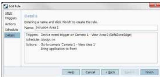
15. Once completed, the process needs to be repeated for all other detection zones configured. In this example, the second event (Intrusion Zone 2) will activate the main camera image (View Area 0) as shown in the summary below.
