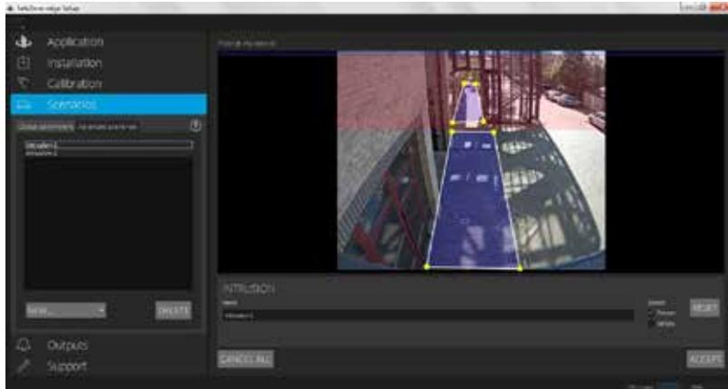
3. The Axis cameras then needs to be registered onto the Video Management Software, ACS. It is important that the View Areas are configured before this step as they need to be added as individual camera streams during this process. ACS is able to automatically detect View Areas configured in the cameras and will display them as available camera channels during its auto search. View Area 0 is always the complete camera view and View Areas 1 and above are for the user defined views.
