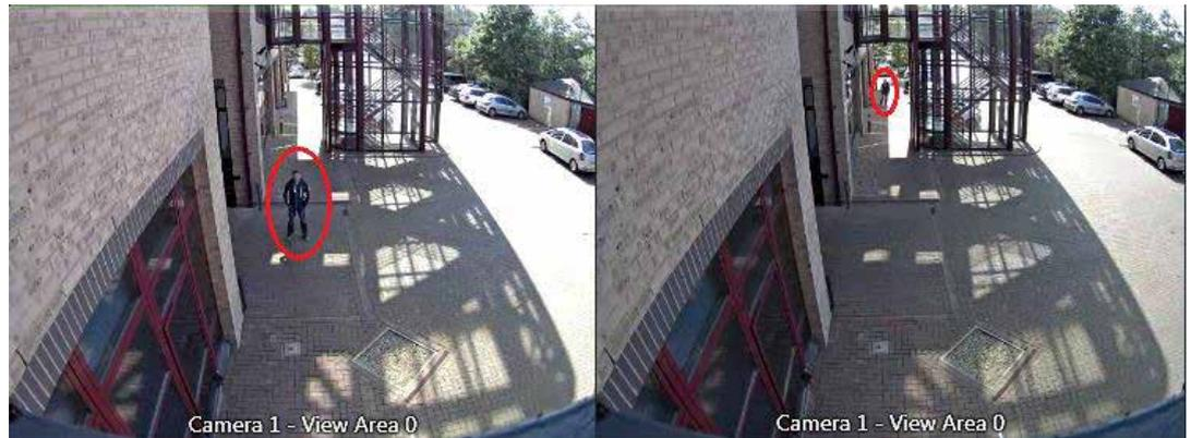
For this reason, many security system designs still require that when an automatic detection occurs, the object still fills a minimum proportion of the operators screen to enable accurate secondary visual verification of the event.
