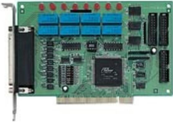
The CitySync JGIO-30 relay card is the contact interface between the ANPR software and external components.
