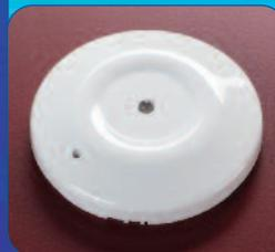
A light-weight remote indicator specifically designed for use with AlarmSense detectors. Measuring just 20mm high and 80mm diameter, two pairs of keyholes are provided - one for 50mm and one for 60mm fixing centres.
