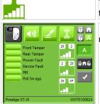
The device signal strength meter details the strength of signal between the device and the receiver, or the device and another device on the system which it is hopping through.
