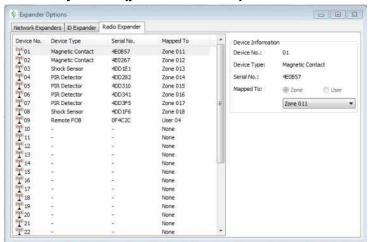
The Radio Expander page shows all of the Radio Devices on the system, the Device Type, The Serial Number and to which Zone/User the device is mapped. Not applicable to *Premier Elite™* V2.xx panels and *Ricochet™* MT2
