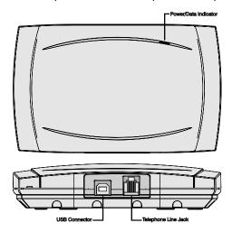
Figure 1. USB-Modem Indicators and Connectors
