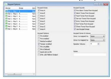
Select the keypad by clicking on the relevant keypad in the left hand panel.
