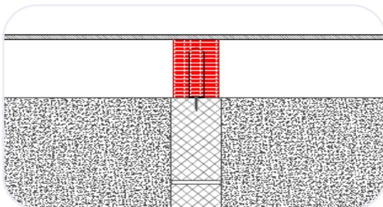
**NVFB Fixed between Mineral Fibre Insulation**
