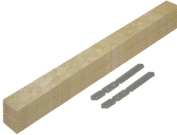
Tested in accordance with BS 476:Part 20, **TENMAT** NVFB Non-Ventilated Fire Barriers provide up to 2 hours fire protection for vertical rainscreen/cladding cavities. The NVFB Non-Ventilated Fire Barrier is used for preventing fire penetration to adjoining compartments within external cavities in a vertical situation for specified periods of up to 2 hours. They are manufactured to suit cavity widths and are held in place by a combination of compression and multi purpose brackets.
