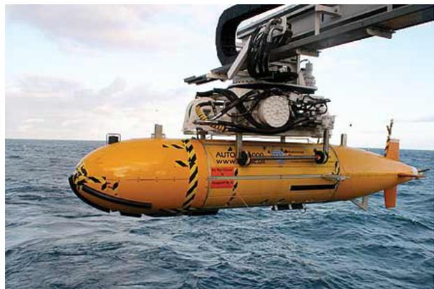
The Autosub Autonomous Underwater Vehicle uses purpose-designed Magnet Schultz technology to release abort weights in the event of a fault. The sub has now completed successful deep sea surveys to depths up to 4600m.
