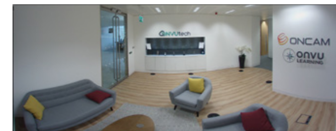
Example 6: optimized panorama from a specialized wall mounted 180-degree camera tilted 20-degrees down with on-board dewarping correction
