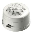
There are two heat detectors in the XPander range, designed to suit a wide variety of operating conditions. A Static Heat Detector (CS) which responds only when a fixed temperature has been reached and a Rate-of-Rise Detector (A1R) which has a fixed upper limit, but in addition, measures the rate of increase in temperature.
