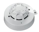
The XP95 Optical/Heat Multisensor Detector contains an optical smoke sensor and a thermistor temperature sensor whose outputs are combined to give the final analogue value.
