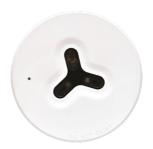
The innovative design of the Soteria Dimension Optical Detector differs from standard fire detectors, having no chamber and being flush mounted. A new optical sensing technology is used to detect smoke particles outside the detector housing. A combination of Infra-Red (IR) LEDs and photo-diodes identify smoke particles, detected just below the detector housing and initiates an alarm
