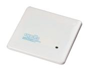
The XP95A Priority Switch Monitor Module is designed to monitor the state of one or more single pole, voltagefree contacts and to report this status to Apollo-compatible analogue control equipment. It can also place a signal on the loop to provide early warning if a device such as a pull station is operated.
