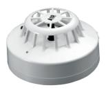
The Series 65 Heat Detector monitors temperature by using a dual thermistor network which provides a voltage output proportional to the external air temperature.
