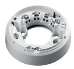
The Orbis Heater Base is designed to be used in cold climates where environmental conditions could result in either icing or condensation affecting the operation of detectors. It is recommended that the heater base be used in conjunction with either a Waterproof Base Cover or Deckhead Mounting Box to minimise moisture ingress.
