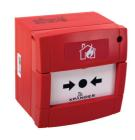
The XPander Manual Call Point is compliant with EN 54-11. It is wireless and is powered by two independent packs of three AA alkaline batteries with a typical five-year life.
