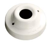
The Marine Intelligent Base Mounted IR³ Flame Detector is designed to protect all indoor areas, even in dirty or smoky conditions, where open flaming fires may be expected. The detector has three IR sensors that respond to different IR wavelengths to discriminate between flames and spurious sources of radiation.
