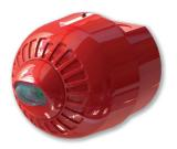
Conventional wall mounted Visual Alarm Devices are available with a white and red flash colour. The white flash variant has an EN 54-23 approved coverage pattern of W-3.1-11.3, whereas the red flash variant has a coverage pattern of W-2.4-7.5.
