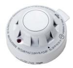
The XP95 I.S. Ionisation Smoke Detector uses a low activity radioactive foil to detect fires by irradiating the air in the smoke chamber and causing a current flow. If smoke enters the chamber, the current flow is reduced, leading to an alarm.
