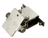
The Flame Detector Bracket is an optional accessory for Flame Detectors. It is a stainless steel mounting bracket adjustable in two axis. Not suitable for Base Mounted Flame Detectors.
