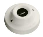
The Marine Series 65 Base Mounted UV Flame Detector is designed to protect enclosed indoor areas where open flaming fires may be expected. The detector has a fast acting response to flames up to 25m away and is equipped with a single UV sensor with a narrow spectral response in order to discriminate between flames and most spurious sources of radiation.
